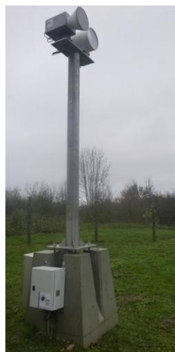
**Figure 11b.** The scintillometer in Les Avenelles catchment (source: ORACLE instrumentation report).
