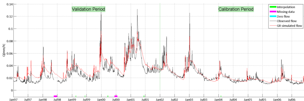
Figure 7—5. Observed and by GR4H simulated hydrograph calibrated on period S2 of catchment H8042010 – Epte at Fourges – 1386 km 2 .
