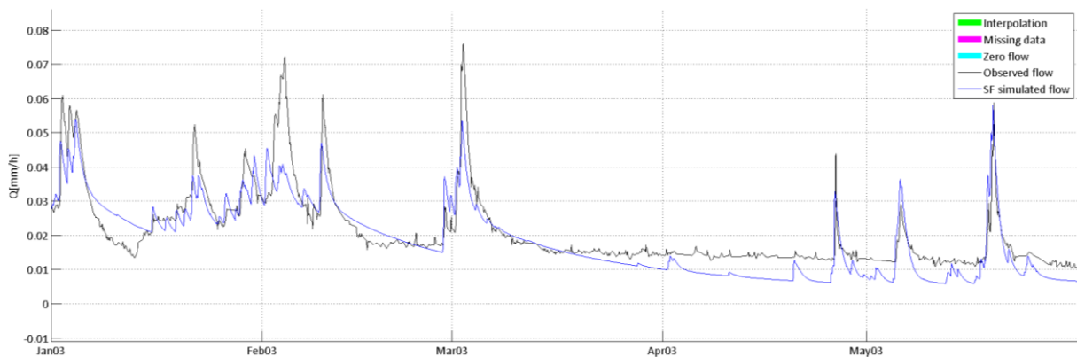
Figure 7—14. Hydrographs of catchment H4223110 – Remarde at Saint-Cyr-sous-Dourdan – 151 km 2 , a zoom of January through June 2003 with model results (SF07) in validation. An example of unnatural recession.
